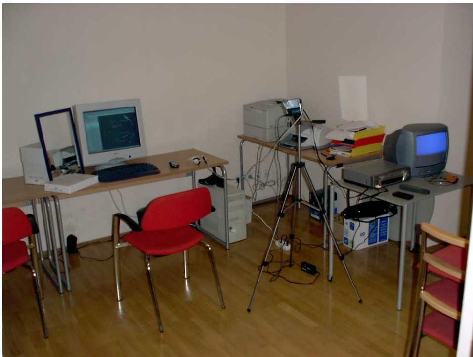
Figure 9.3: A simple usability test with a single video camera. A mirror is used to capture the user's facial expressions.
