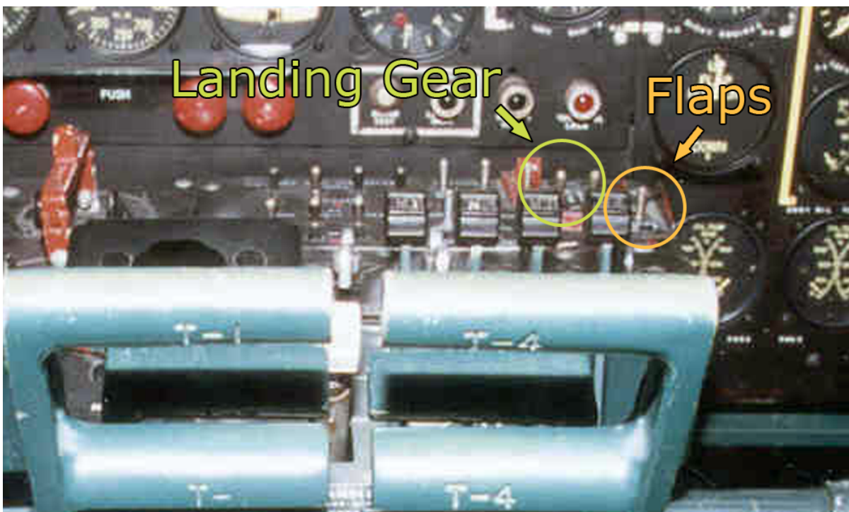
Figure 2.29: Close-up of the cockpit control knobs of a B17G Flying Fortress. The landing gear and flaps control knobs are identical and are very close to one another. [From USAF [2006], image believed to be in the public domain.]
