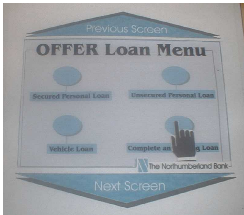
Figure 7.4: Paper prototype 2 for a customer information terminal. [Image used with kind permission of Cliff Brown, Northumbria University.]
